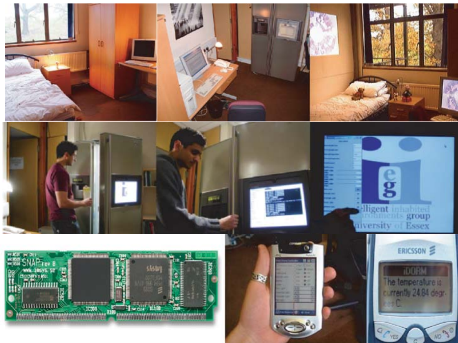
Fig. 1. The iDorm general overview (top row). The iFridge, a refrigerator with internet capabilities hosting the intelligent agents to control the iDorm (center row). Different possibilities to interface the intelligent agent: SNAP controller (left), PDA interface (center), mobile phone interface right (bottom row).
